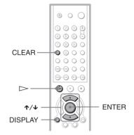
**1** Press DISPLAY twice during playback (when playing a DATA CD, press once). The Control Menu appears.
